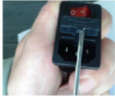
1. Turn off the power and pry up the fuse groove with a screwdriver;
