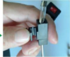
3. Remove the damaged fuse with a screwdriver
