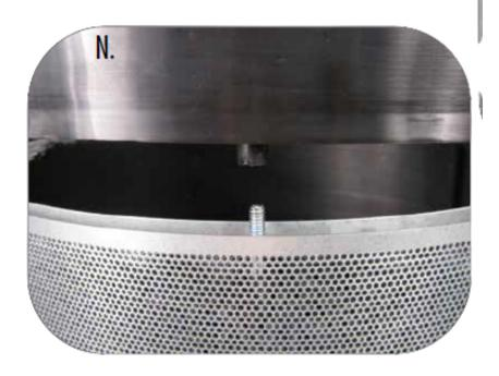
After discarding the old saturated carbon, use the provided funnel to pour the fresh activated carbon into the unit. For proper placement, align and place the funnel on the 3 metal posts (see box N).
