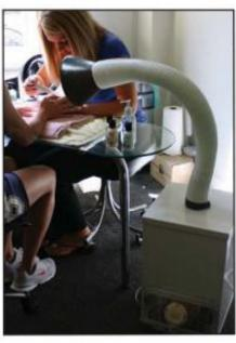
Source-capture systems, as the pictured here from Aerovex Systems, protect the breathing zone of the tech and the client.
